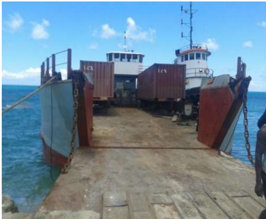
Figure 7: “1473” on a previous voyage showing the bow ramp arrangement Photo: Owner
