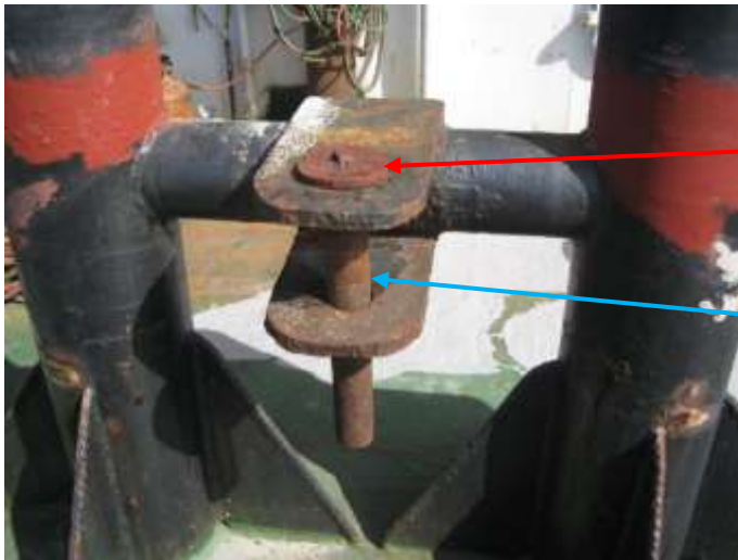
Figure 9: The towing pin mounted on the original towing bits. Photo: ADOMS
